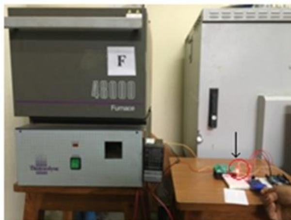
Fig. 7 (c): Alarm (Red LED) ON when Invalid (Blue) card is detected
