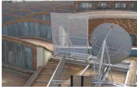
Figure 3 a: Scheffler Reflector being used as a Solar Cooker to Cook Food by Concentrating the Sunlight
