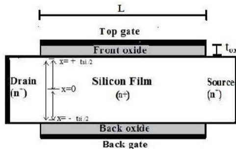
Fig. 1 Cross-section of DG JL MOSFET
