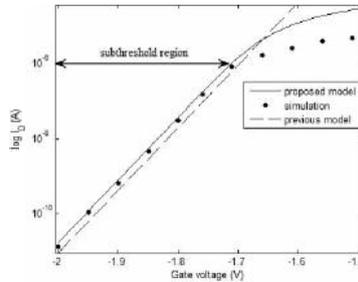
Fig. 7(a) Transfer characteristics for symmetrical DG JL MOSFET in logarithmic scale for the proposed model and previous research model compared with simulation (symbol) results.
