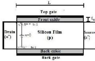
Fig. 3 Cross-section of DG MOSFET
