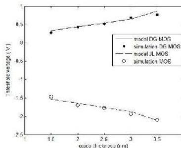
Fig. 9 Threshold voltage comparison between DG JL MOSFET and DG MOSFET for oxide thickness variation for the proposed model and simulation results
