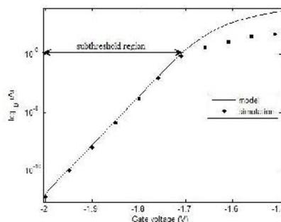
Fig. 5(a) Transfer characteristics for symmetrical DG JL MOSFET in logarithmic scale for the proposed model compared with simulation (symbols) results.
