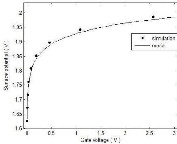
Fig. 4 Surface potential variation with gate voltage for undoped symmetrical DG MOSFET
