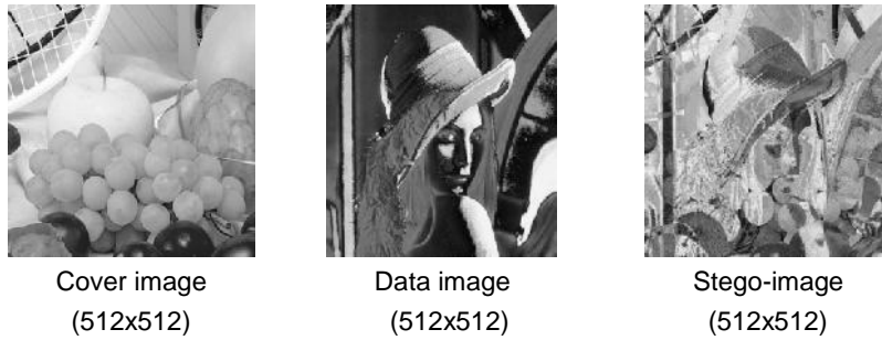
Figure 6: 4-bit & 8-bit XORing methods with same cover image and different size of data image.
