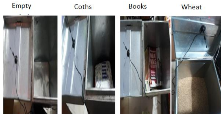
Figure 7: RF Through-Beam System when RF Transmitter Antenna is on Up and RF Receiver Antenna on Bottom of Container
