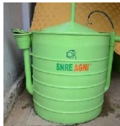
Small bio gas plant to treat 20 to 50 kg
