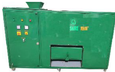
100 kg per day organic waste composting machine Size of the machine depends on the waste to be treated
