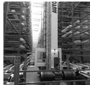
The above picture denotes the stacking system ASRS for Fabric Rolls. Shuttle and Conveyer
